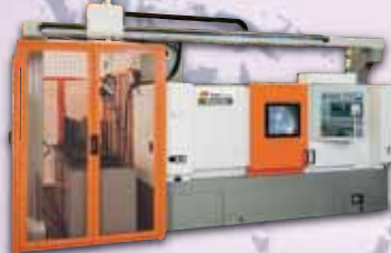
VturnII-26 (Y-axis, C-axis) Gantry robot automation
